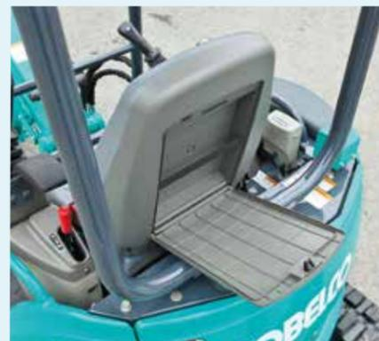
Easy Access to Control Panel and Levers
