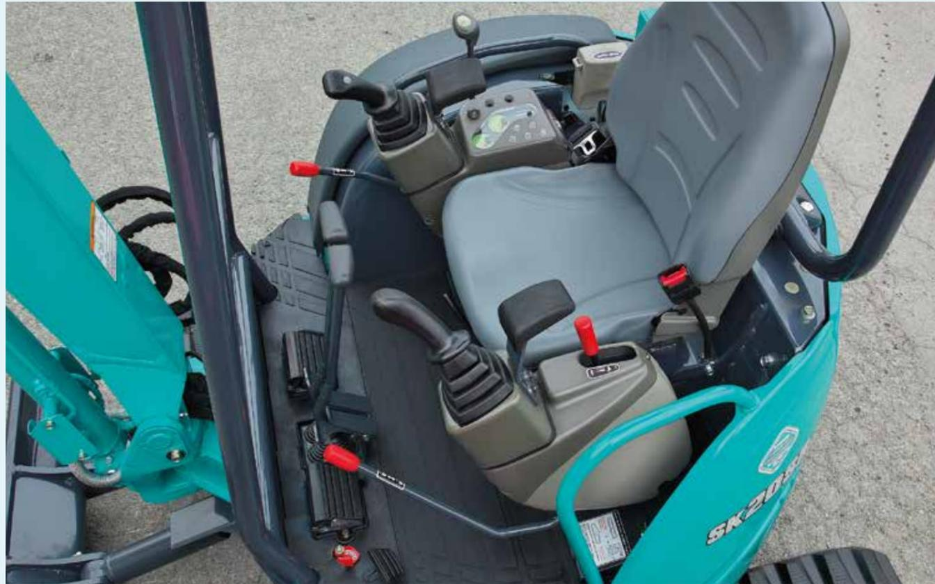
Broader floor space gives operators plenty of foot room. Wide operational space is provided with more room between the left and right control consoles.
